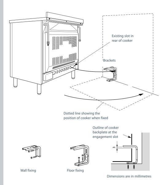
Figure 10 Fitting a stability bracket
